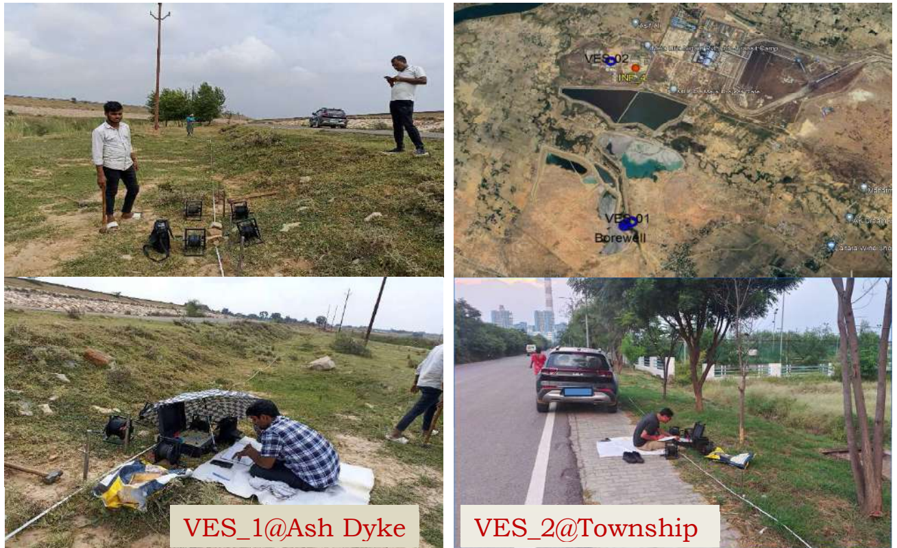
Figure 6.2: Conducting Geophysical Survey (VES Test) at two locations (1) Near Ash Dyke (2) Inside the NTPC Meja Plant.
