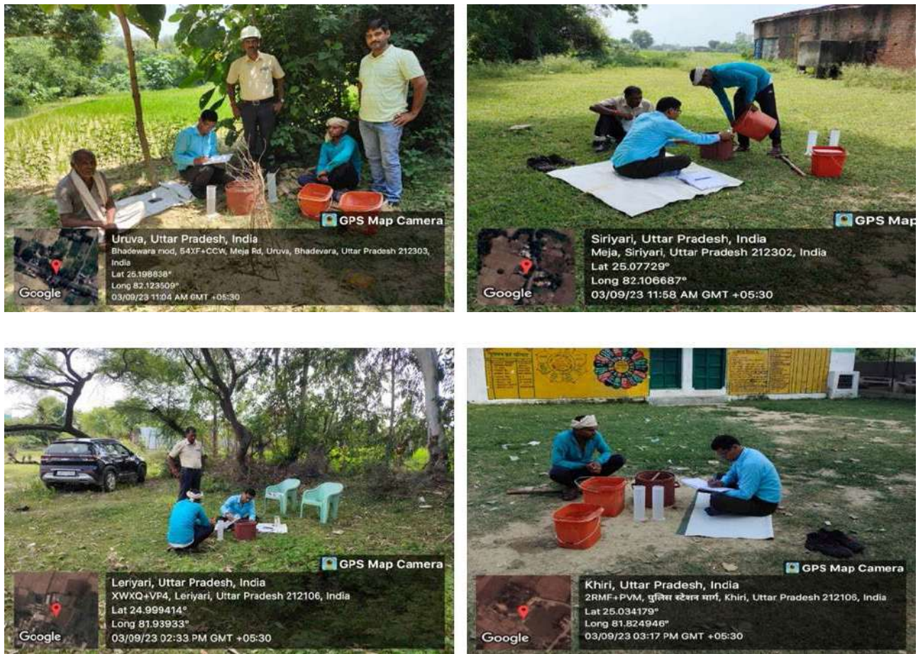
Figure 4.5: The field setup of the double-ring infiltration inside the NTPC Meja Plant and 25 Km radius buffer zone.
