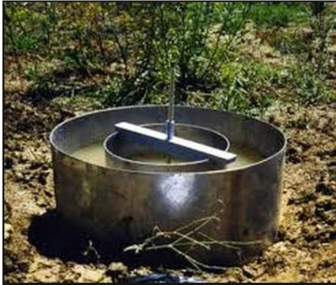
Figure 4.4: Field set up of double ring infiltrometer
