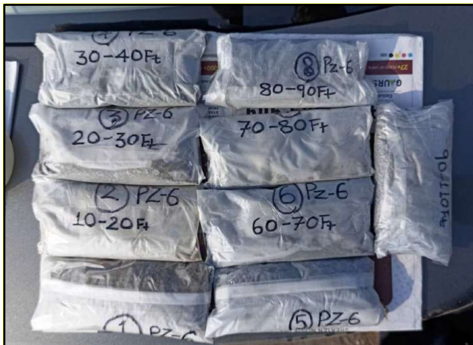
Figure 6.6: Soil/Sediment from drilling samples collected from the newly installed Piezometers at NTPC, Meja
